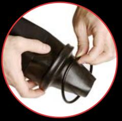
Push the sleeve protective ring (MS) with the larger diameter over the sleeve and the o-ring and click into
