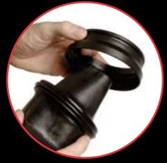
Put the red o-ring slightly lubricated into the provided slot of the sleeve protective ring (MS)
