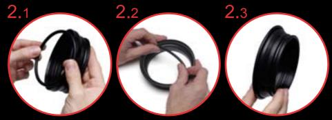
Insert the sleeve protective ring (MS) with the drawn-on o-ring ahead into the latex diving glove and put the diving glove up to the groove over the o-ring in the same way.
